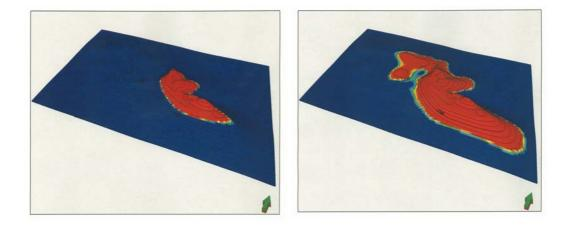
Fig. 11 - Identification of gas losses – gas saturation after simulating the correct storage operation in comparison with gas saturation after simulating the historic, real and incorrect storage operation (red = gas, blue = water)
