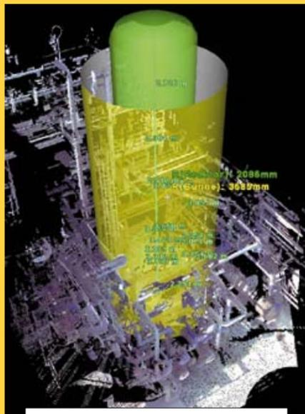
Laser scanning point cloud with reactor disturbing edges model for quick collision check
