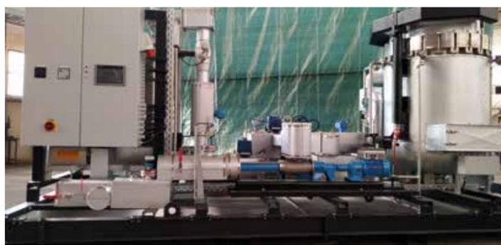
Customers can now test their own lube oil formulations on site with EDL's portable LEPD pilot plant. The plant was manufactured by TAF.
