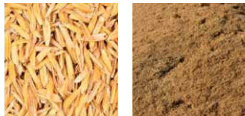
The waste product - unground and ground rice hulls - are further processed
