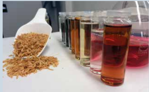
Several sodium- and potassium silicates, ash and carbon adsorbent suspensions
